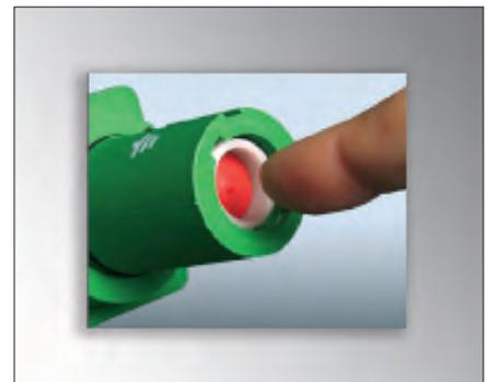
The drain protected connector features a patented double protection to prevent accidental touch of the drain contact under load. The drain contact must be unlocked supplying uniform pressure on the entire Teon part (by means of the female connector).
