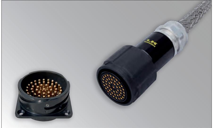
**LKA 48/6** was designed to connect speaker clusters to their amplifiers utilizing the least possible number of cables, up to 24 speaker channels using a cable with a 4mm<sup>2</sup> section, Eurocable 36N40AD2 or 48N40AD2. Additionally, there are 2x AES/EBU channels for laser pointing and inclinometer control, and the LKA 48/6 features a mesh cable gland as standard for maximum durability.
